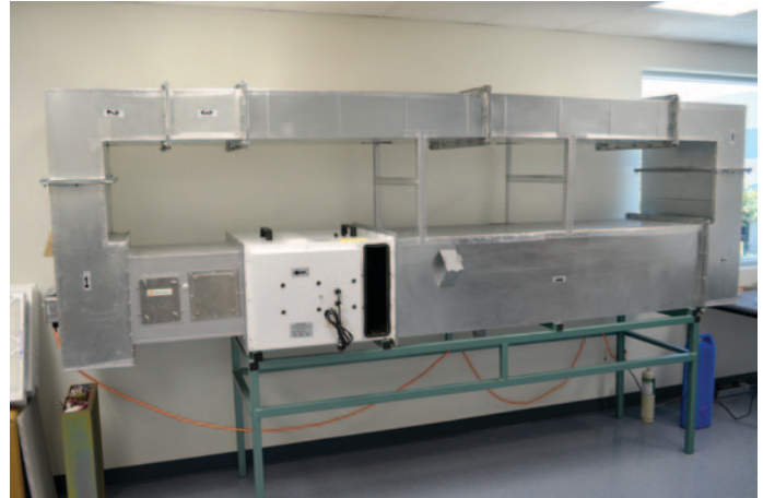
Through Duct Test Chamber - State of the art computerized monitoring allows for adjustable airflow, scheduled monitoring of CO 2 , VOCs, Ozone, and more.
