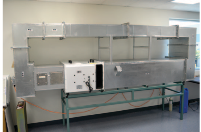
Through Duct Test Chamber - State of the art computerized monitoring allows for adjustable airflow, scheduled monitoring of CO 2 , VOCs, Ozone, and more.
