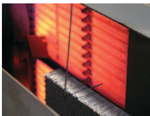
Patented application uses nano-sized Anatase TiO 2 infrared-bonded to honeycomb aluminum substrate.
